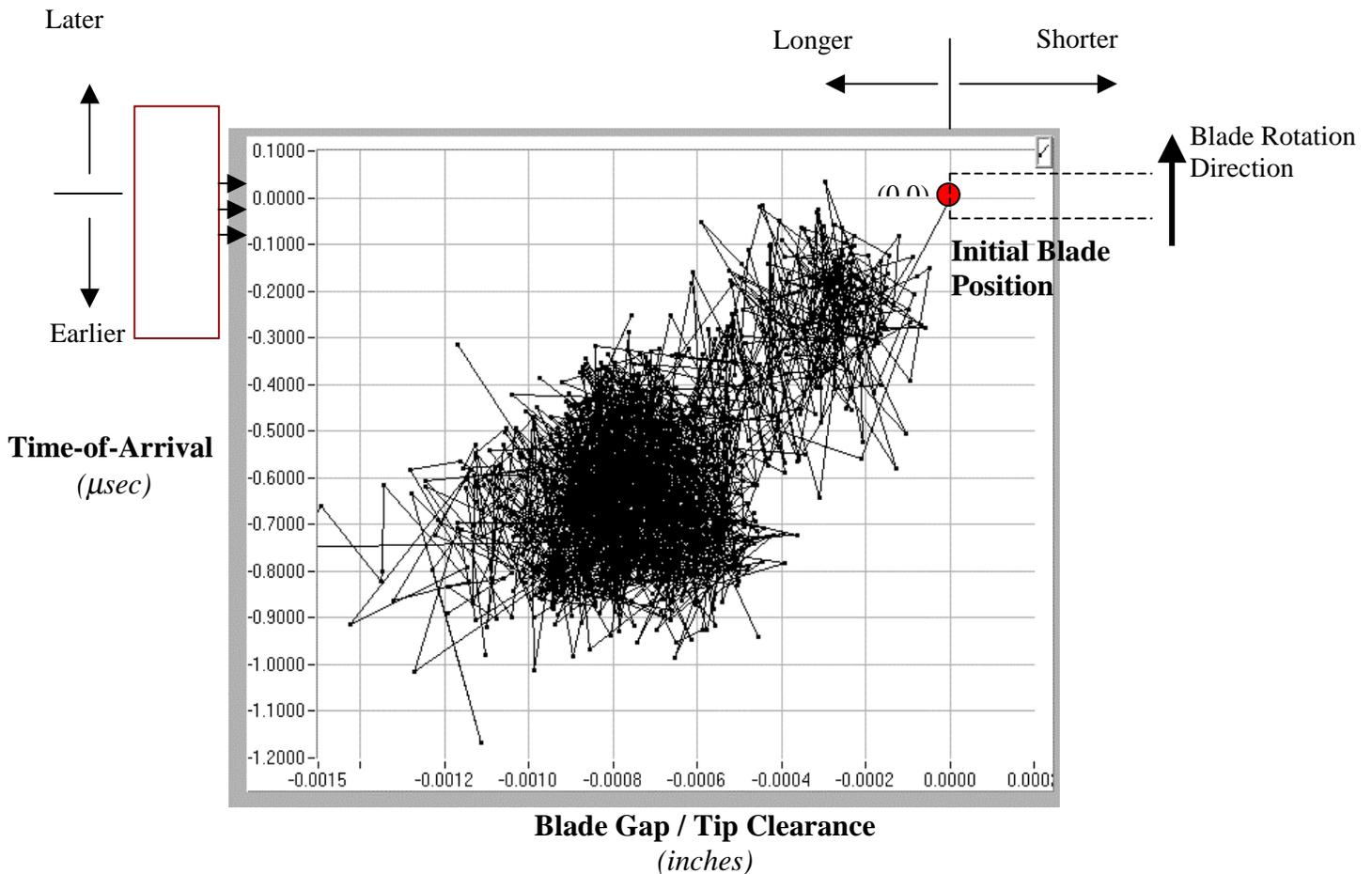
**Fig. 8 – Blade Movement Plot During Spin Test of Large Fan Showing Time-of-Arrival on Vertical Axis and Blade Gap on Horizontal Axis**
