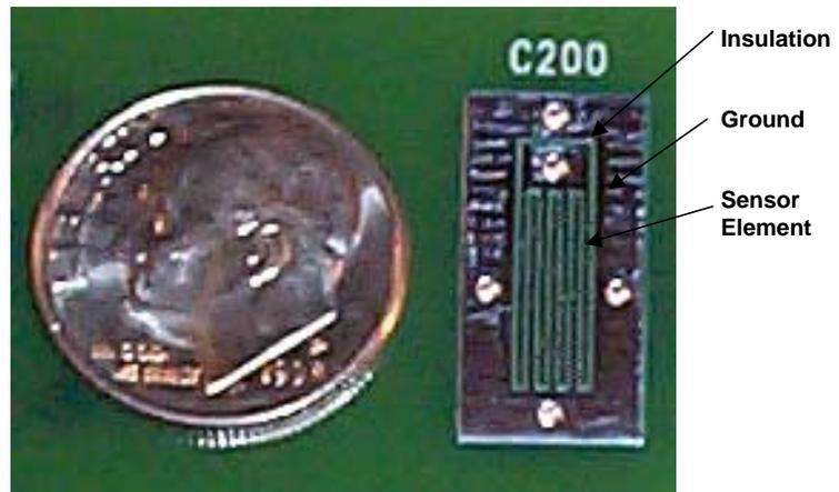
**Fig.4 - Small MasterPlex probe for bladed wheel.**
