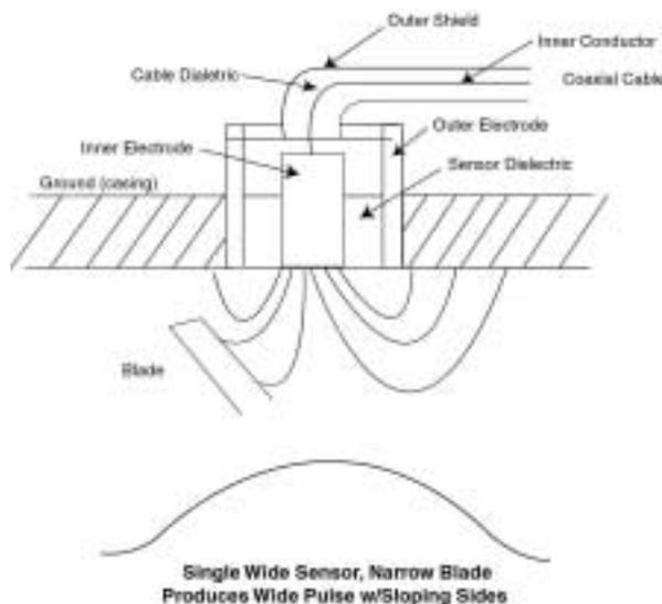
**Fig 1 - Example of Low Resolution Output from a Capacitive Measurement Using a Typical Wide, Single Element Sensor**
