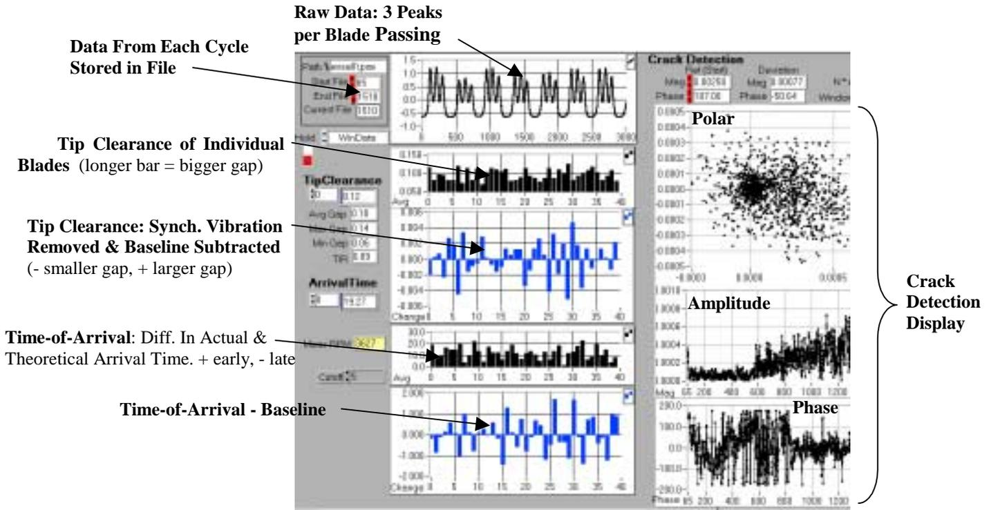
**Fig. 7 – Screen From ExSell Acquisition System Showing Raw Signal, Tip Clearance, Blade TOA and Crack Detection From Spin Test of Large Aircraft Fan.**
